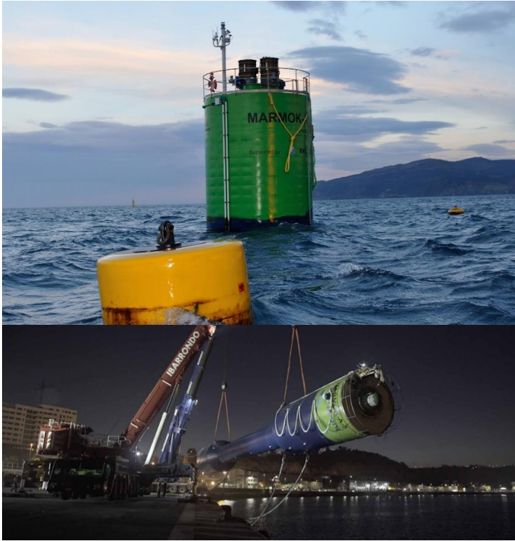
MARMOK-A5 OWC-WEC operating at BIMEP
