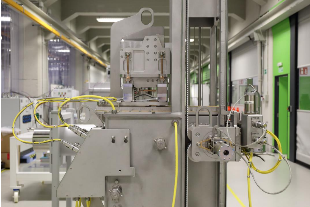
Jules Horowitz Reactor Hot-Cell X-Ray Tomography and Gammametry Bench (@ IDOM Integration Hall)
