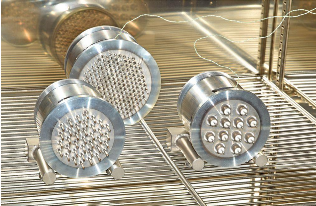
Qualification models of Electrical Feedthroughs for the ITER Vacuum Vessel first confinement barrier
