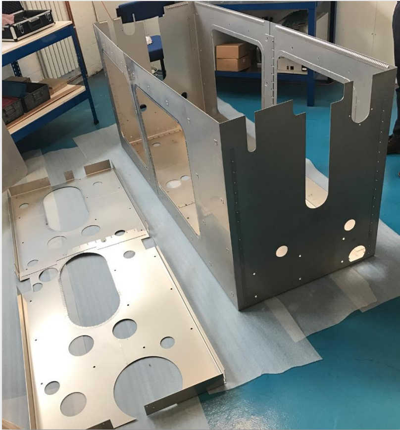
Warm Magnetic Shield MuMetal, 2m wide
