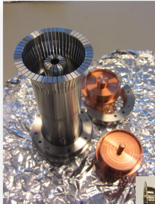
RF Power Lines Ambient to Cryogenic
