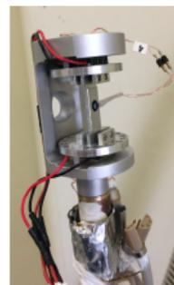
"Huginn: A Peltier-based sub-cryostat for neutron scattering",
